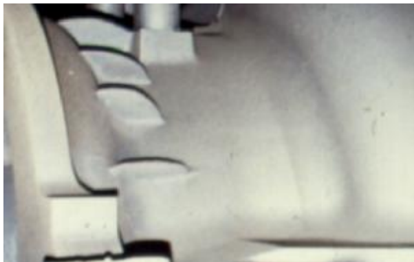
Fig.10. Close up view of ingate area of figure 8. No erosion even though the pouring time was less than one minute.
