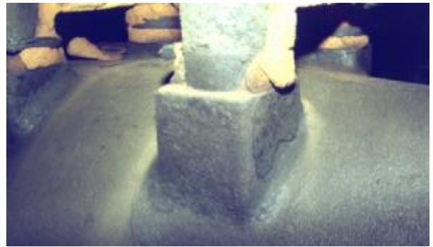
Fig.23. Double skin on an ingate.
