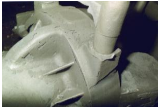
Fig.18. A close up view of Figure 16. Notice how the severity increases adjacent to the ingate areas.
