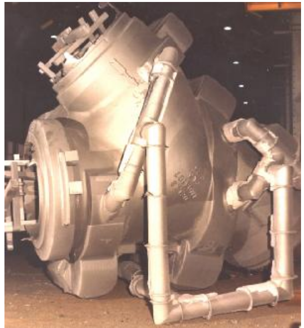
Fig.12. "Y" Connector casting, 18 Tonnes, Chromite facing sand. Pouring time 47 seconds.
