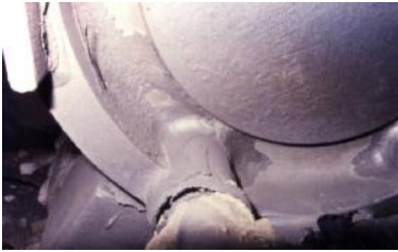
Fig.19. End case casting. Severe double skin around ingate.
