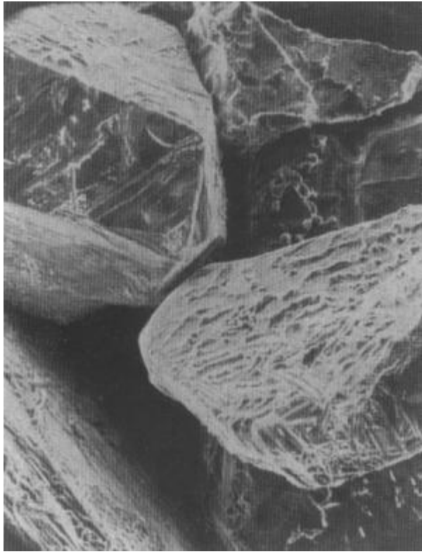
Fig.37. Resin bonded chromite, fired at 1300C. Note crystallographic planes.
