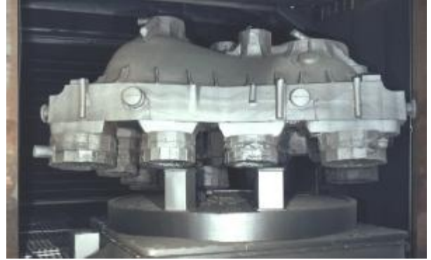
Fig.11. Turbine casting, 40 tonnes, chromite facing sand. Pouring time 90 seconds.
