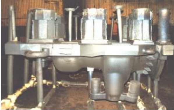
Fig.8. Steam turbine casing, 15 tonnes Cr/Mo steel, Chromite facing.
