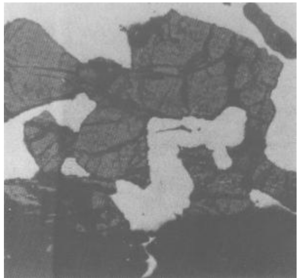
Fig.32. The defect X60 Slag and chromite dark gray colour. Metal light grey colour.
