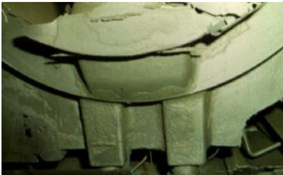
Fig.21. Example of a very difficult to remove double skin.
