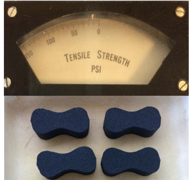
Gauge on tensile testing equipment and standard AFS tensile specimens
