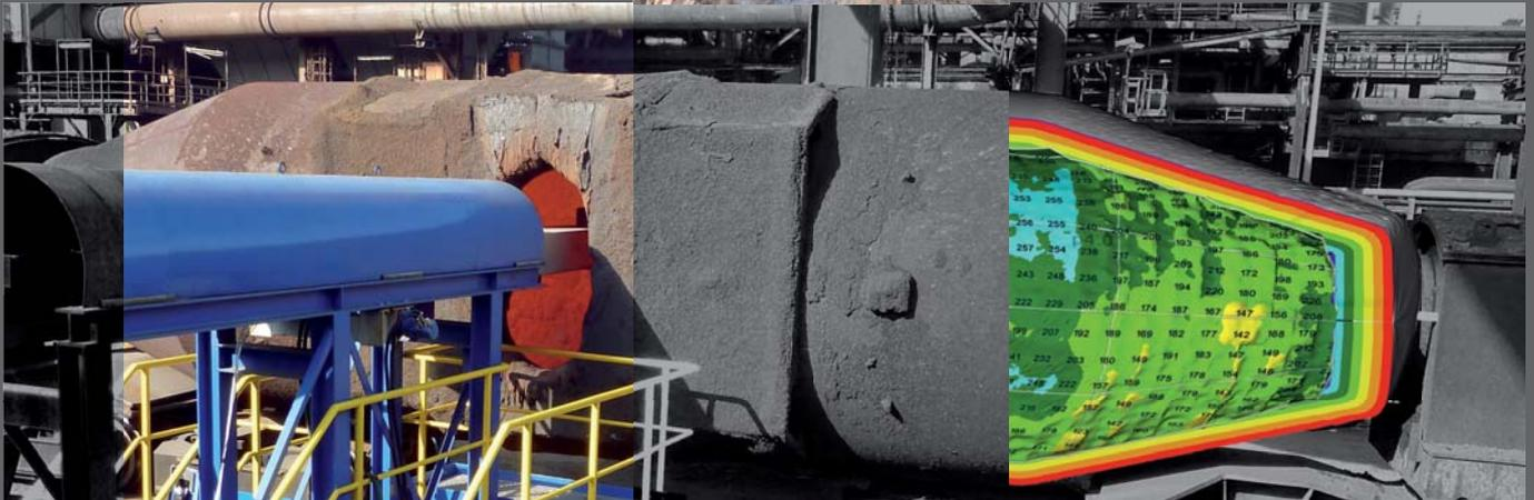
3D-Laser Profile Measurement for Refractory Lining Thickness in hot Torpedo Ladles.
