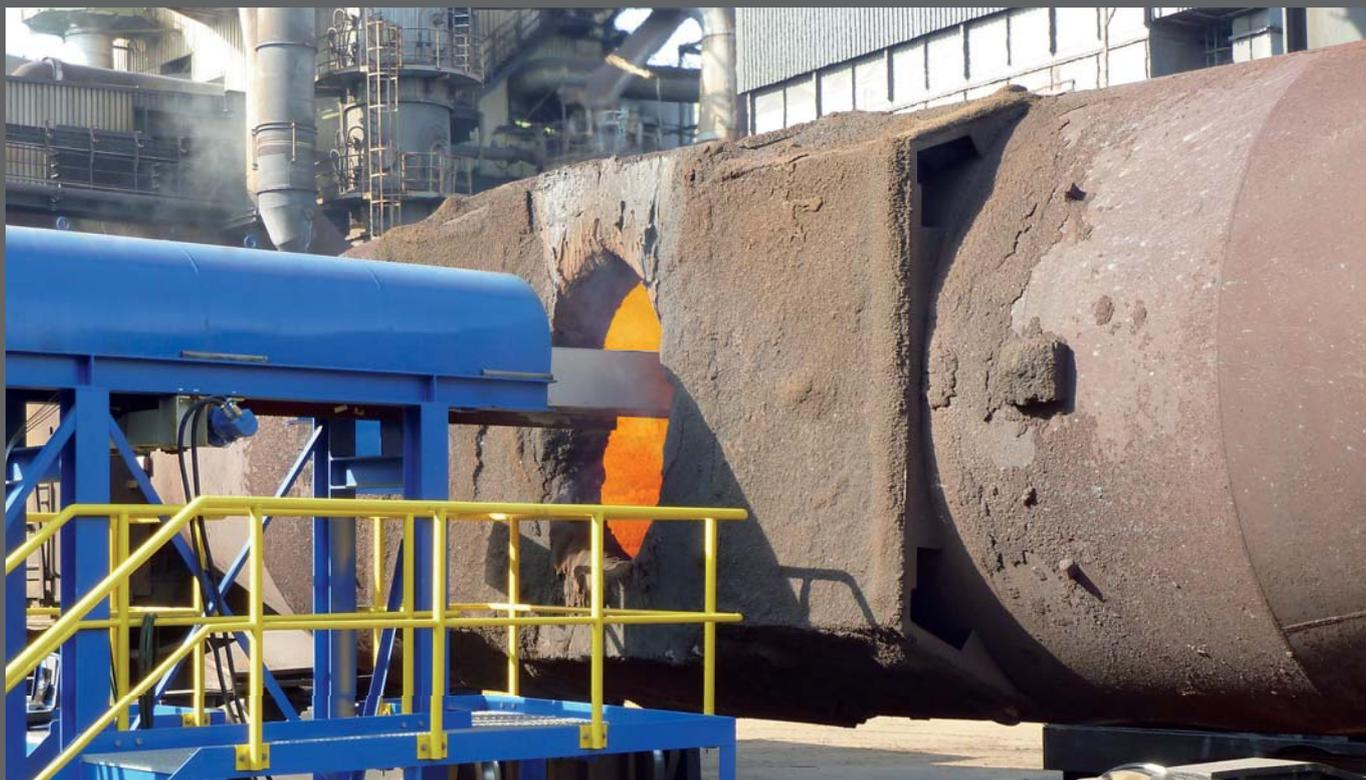
Complete measuring system consists of the laser, manipulator, cooling and evaluation systems.
